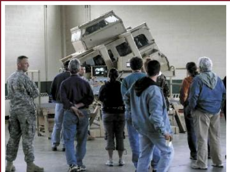
Sgt. Jefferey Jordan, 12th Civil Support Team, orients local civilian healthcare professionals to the HUMVEE Egress Assistance Trainer. The HEAT allows Guardsmen to safely experience and evacuate from a simulated vehicle rollover.
