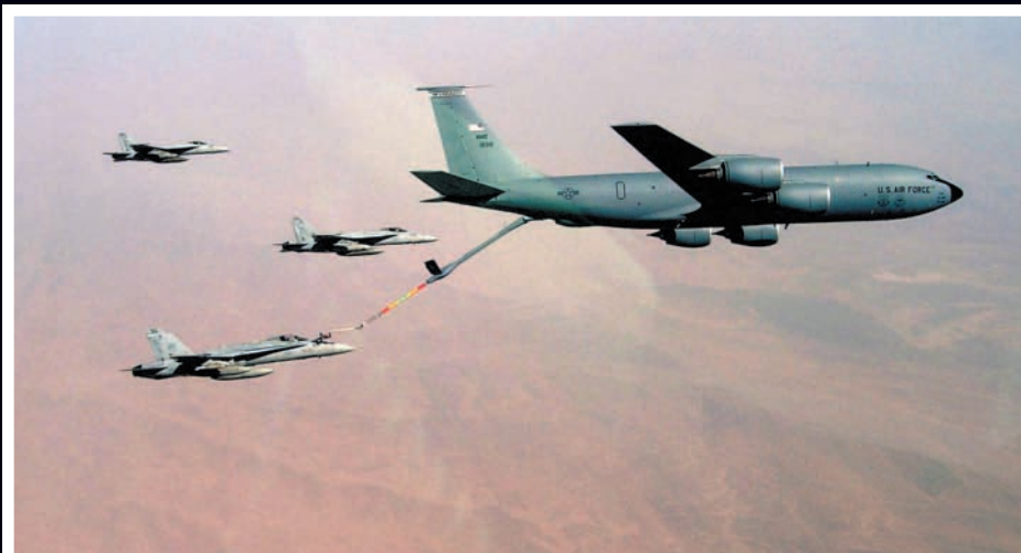
An F/A-18C Hornet refuels from a KC-135R Stratotanker aircraft while two F/A-18E Super Hornets fly alongside during flight operations above Afghanistan. Photo by Cmdr. Erik Etz
