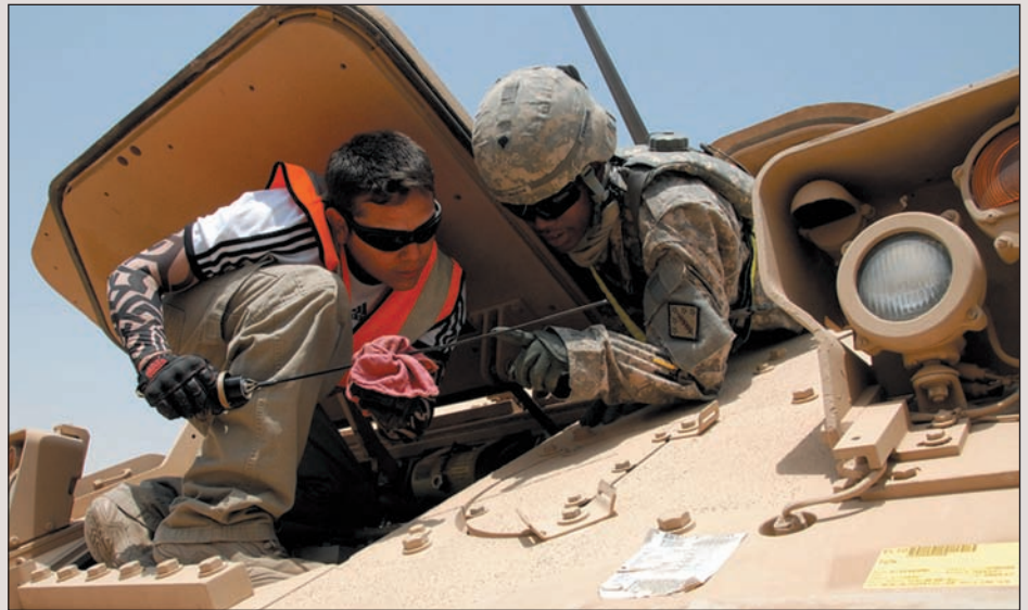
Spc. Jaresha Mason, a chemical specialist with the 44th Chemical Company, inspects the dip stick of a Bradley fighting vehicle held by Juan Ramirez, an American ITT contractor, during a equipment fielding exercise on Camp Arifjan, Kuwait, June 24-25. Photo by Sgt. 1st Class Neil Mitchell
