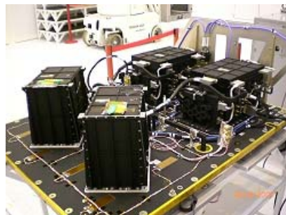
Figure 3 : OSTM/Jason-2 Posidon-3 Instrument
