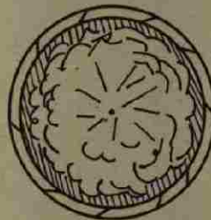
2 IMMEDIATELY UPON DETONATION, CASE EXPANDS TO ABOUT 1\frac{1}{2} ORIGINAL DIAMETER. SHEAR CRACKS DEVELOP
