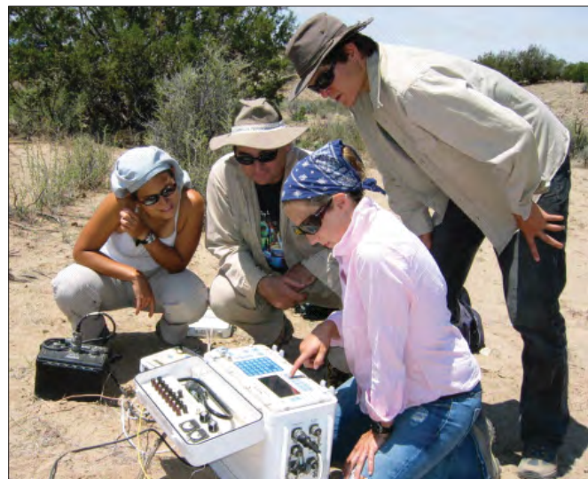
Figure 2. SAGE field camp students acquiring transient electromagnetic data for a groundwater application with Scott Urquart, president, Zonge engineering.
