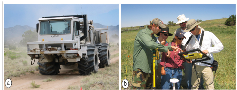
Figure 1. SAGE 2007. (a) Vibroseis source courtesy of ION Geophysical (formerly Input/Output) and (b) students analyze ground-penetrating radar recording with Peter Annan, president of Sensors and Software.
