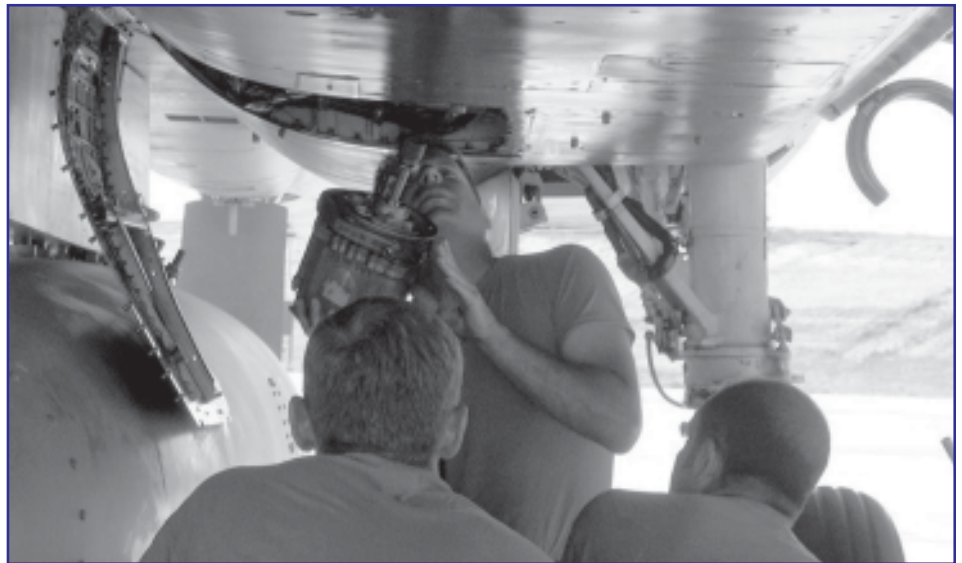
Master Sgt. Jeff Booker installs a hydraulic pump into the belly of an F-15 Eagle.
