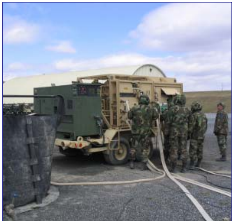
Senior Master Sgt. Robert Sullivan and his team configure a reverse osmosis water purification unit.
