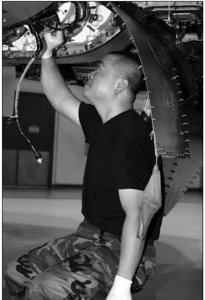
Master Sgt. Wing Ng reconnects cannon plugs on an Eagle.
