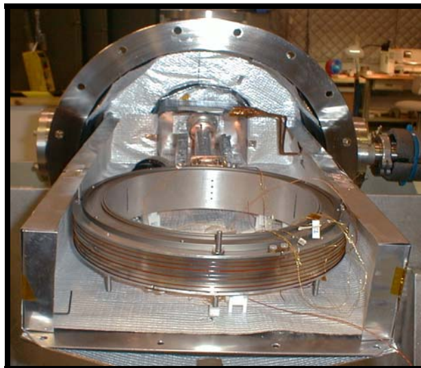
Superconducting magnet installed in test chamber
