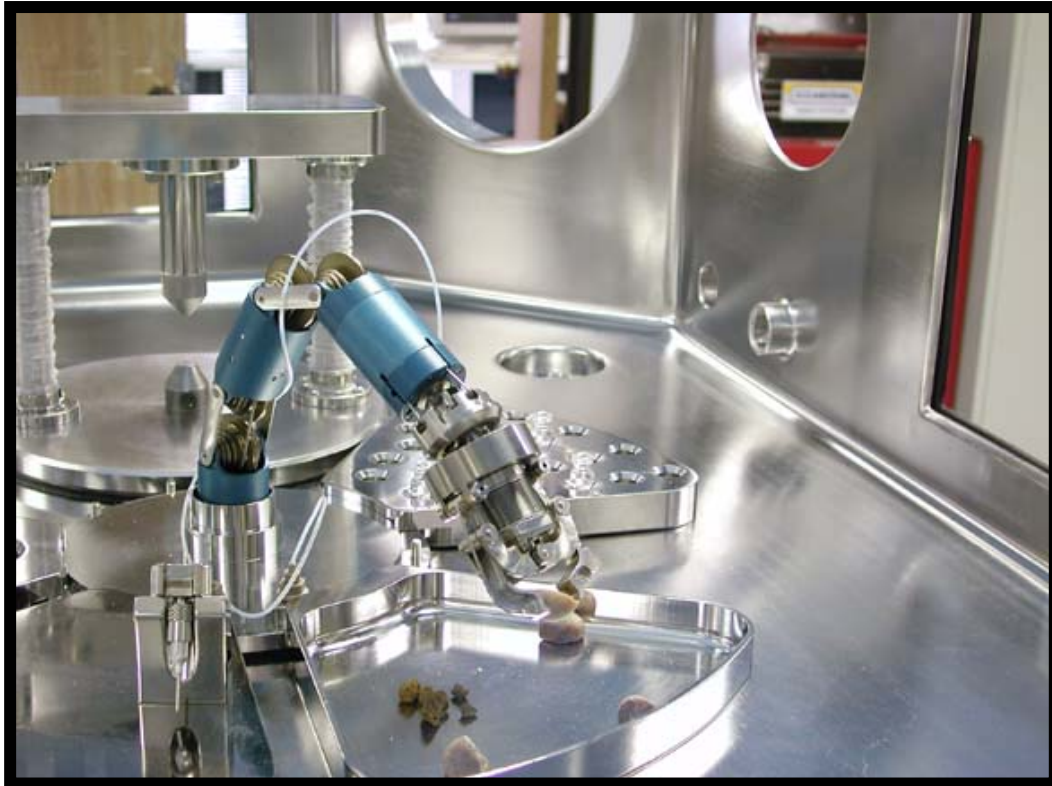
Robotic arm in glovebox
