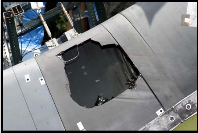
Figure 4. Panel 8L post-test damage.
