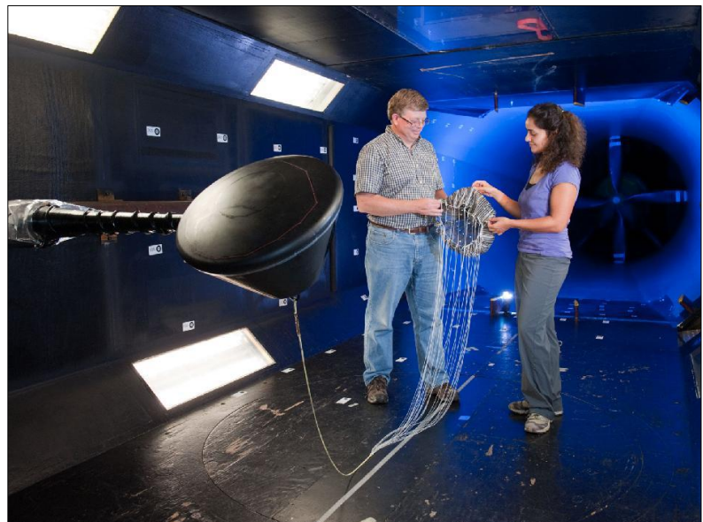
Donn Liddle and Dr. Anita Sengupta in the low speed wind tunnel at Texas A&M University, which is being used for testing of a scale model of the Orion spacecraft and parachute system.
