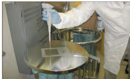
NIOSH researcher collecting a surface wipe sample for possible antineoplastic drug contamination
