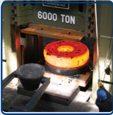
A forged spent nuclear fuel canister seal, being formed on one of the large presses at Custom Alloy Corporation.
