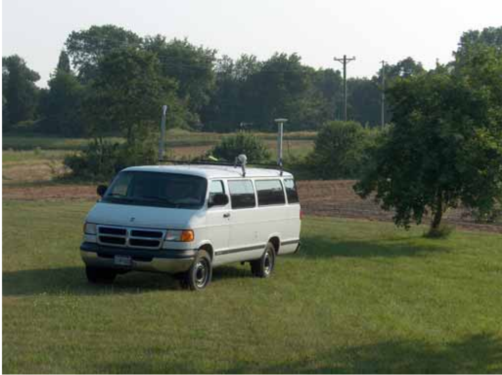
Figure 28. Van configuration used for multipath testing at the Hagerstown GWEN site. In this case, HA-NDGPS marine antenna to van marine antenna is under test.
