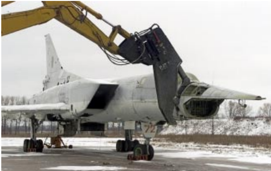
The Heavy Bomber Elimination Program, a U.S. congressional initiative, has provided more than $650 million to Ukraine to scrap its strategic nuclear arsenal in compliance with the START I and Conventional Forces in Europe treaties. This Tu-22MS Backfire bomber is being dismantled as part of that program.
