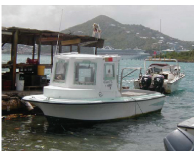
Figure 8.25. Bandit rigged boat - a type of commercial fishing vessel used to fish offshore for deepwater snapper and grouper in the U.S. Virgin Islands and capable of fishing to depths where deep water coral reside. Photo credit: Kojis 2005.
