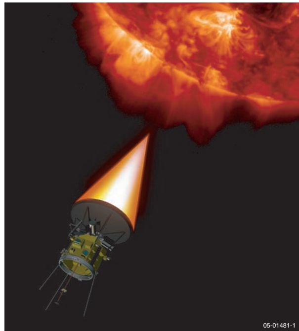
Artist's concept of the Solar Probe, with the glowing cone of the Thermal Protection System pointed toward the Sun inside 0.8 AU.
