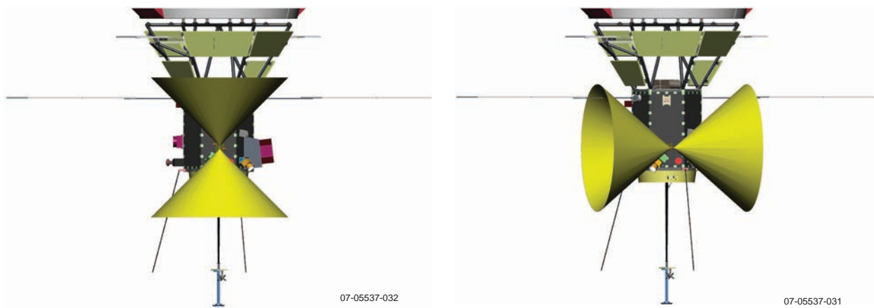
Figure 4-15. EPI-Hi High-Energy Telescope FOV (left) and Medium-Energy Telescope FOV (right).
