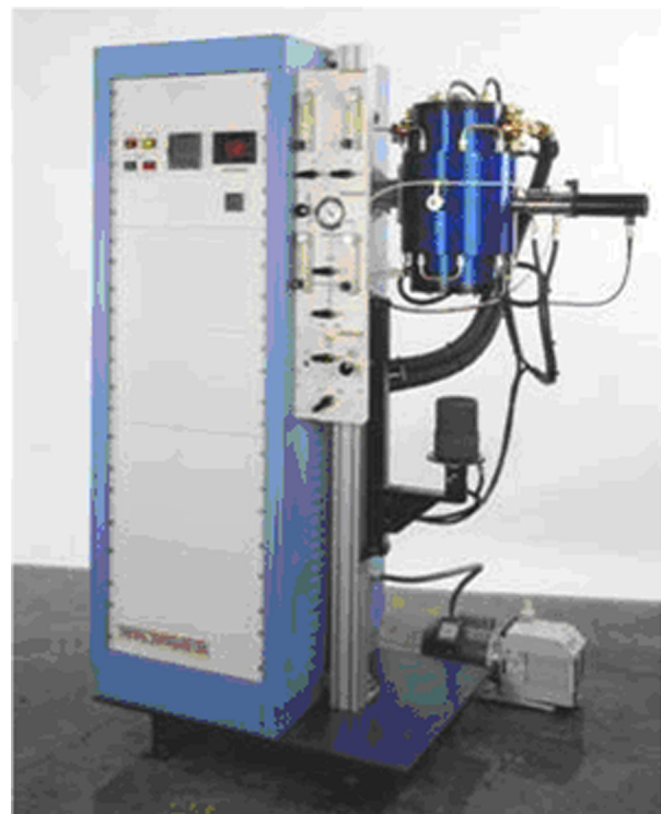
Figure 5-2. APL high-temperature carbon furnace.
