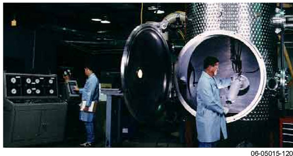
Figure 4-57. Large-scale plasma spraying at Plasma Processing, Inc.
