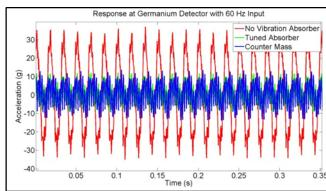
is to use a piston-driven cryocooler to achieve liquid nitrogen temperatures. Piston-driven cryocoolers, can operate unattended, but the microphonic noise induced by the vibrations produced by these coolers causes the resolution of the spectroscopic measurements to severely degrade, making identification of nuclear materials significantly more difficult.
