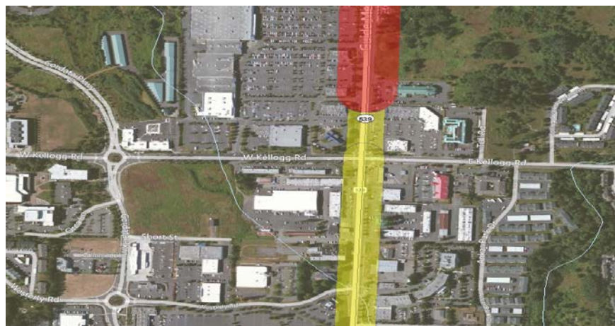
Figure 17. Screenshot of Output from WSDOT's "Potential Area of Noise Effects" GIS model. Different Line Widths Indicate Different Traffic Speeds and Volumes.
