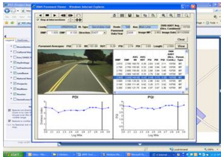
Figure 3. Screenshot of the SCDOT Project Screening Tool displaying a road segment's Pavement Video Log. The charts and graphs show the Pavement Quality Index (PQI) and Pavement Distress Index (PDI) of the roadway.
