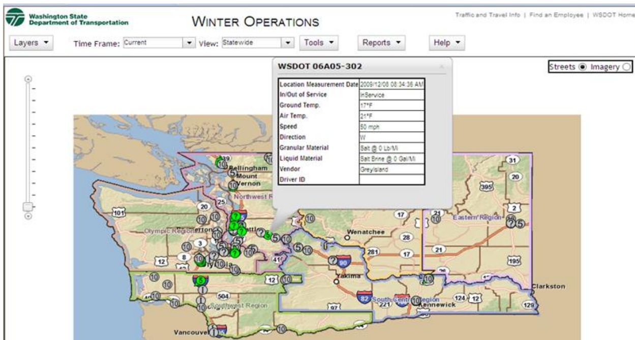
Figure 16: WSDOT's Maintenance Operations System (formerly Winter Operations) shows live information collected from plow trucks. Staff is working on upgrading the system and collecting data from other types of maintenance equipment (such as mowers, line painters, and vacuum trucks) Source: WSDOT
