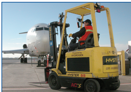
Fuel cell forklifts are safely moving goods in airports and distribution centers across America.
