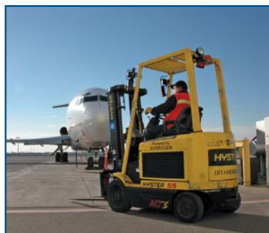
A hydrogen fuel cell forklift
