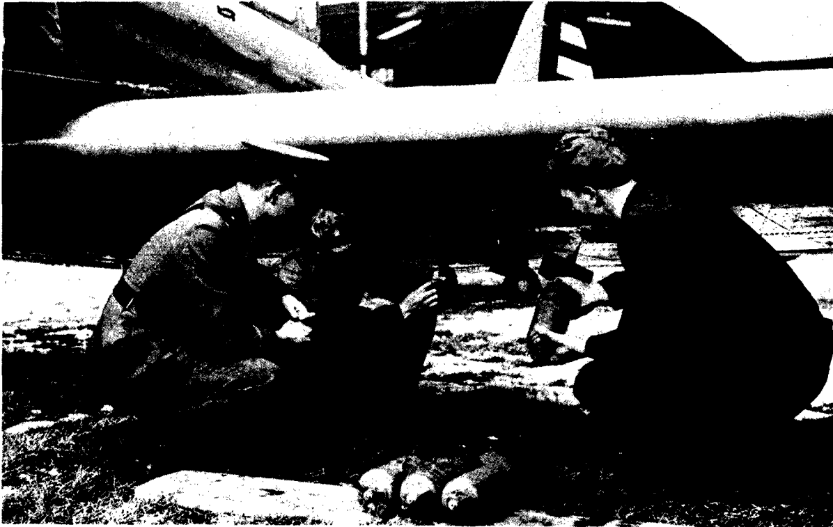
FUZING AND LOADING BOMBS ON A-17 AEROPLANE
