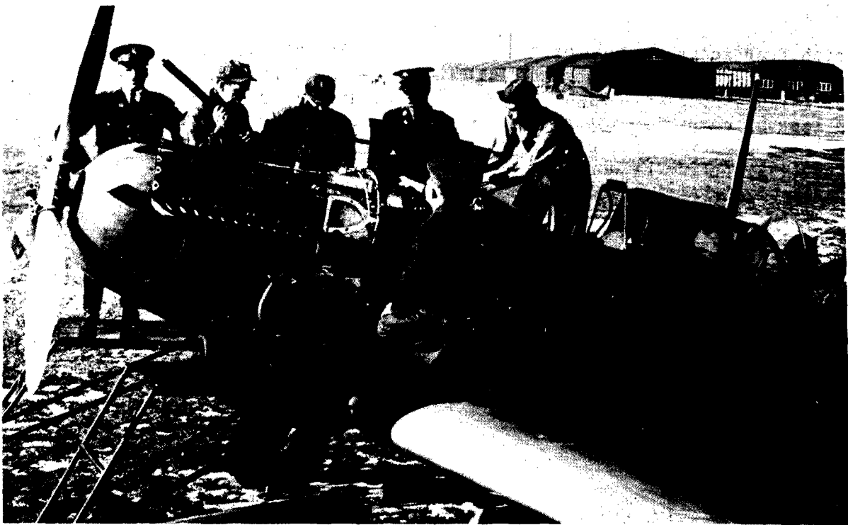
MACHINE GUN INSTALLATION ON TYPE PB-2 AEROPLANE
