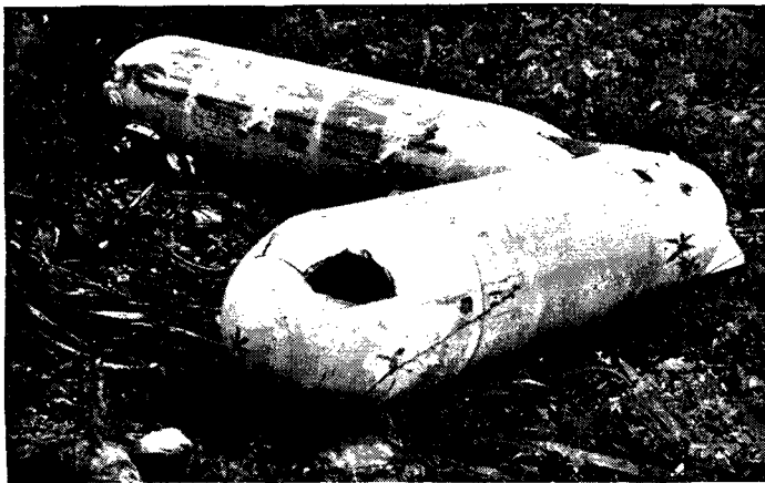
These wooden belly tanks for Japanese planes were found near the Munda airfield after it was taken by American troops. The tanks are of good design and light construction but vulnerable to 50 mm fire.
