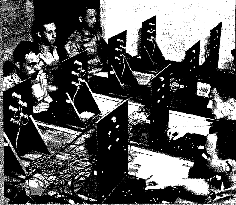
Another reaction time test requires students to manipulate four buttons according to a combination of flashing red and green lights, so as to extinguish a white signal light at top of the panel. A clock records total seconds needed to put out the white light 50 times.
