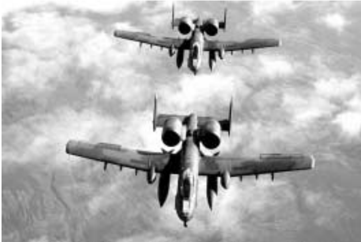
The A-10A features a large gun, armor, high load capacity, long loiter time, and a wide combat radius for close air support.
