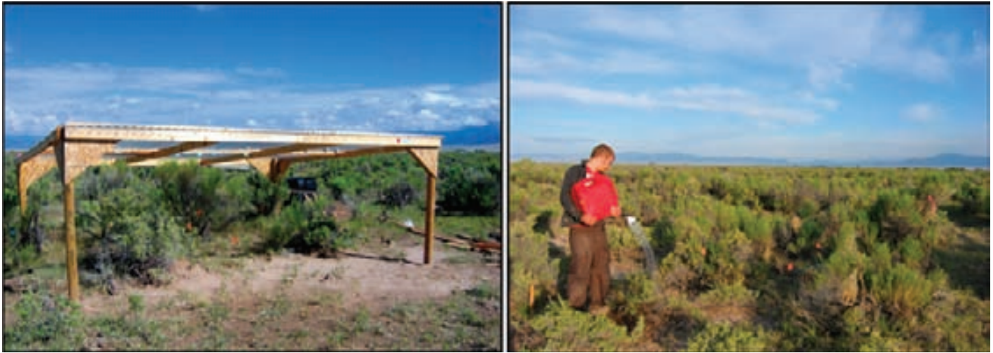
Figure 2: The rainfall manipulation experiment compared control plots receiving ambient rainfall with one of two treatments: (a) decreased rainfall using rain-out shelters and (b) increased rainfall through addition of rain captured by shelter roofs. (Courtesy of Julie Kray)
