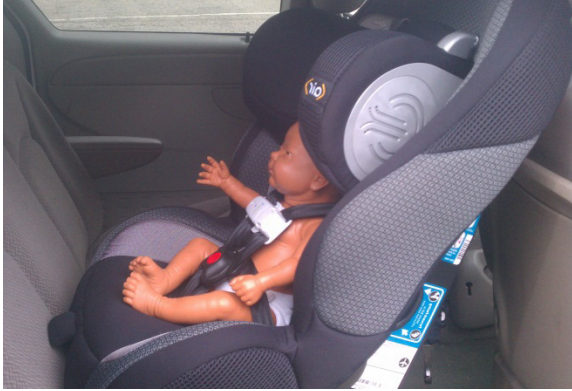
Figure 15a: Newborn (3.4 kg) in a rear-facing Safety 1st Complete Air 65 convertible seat
