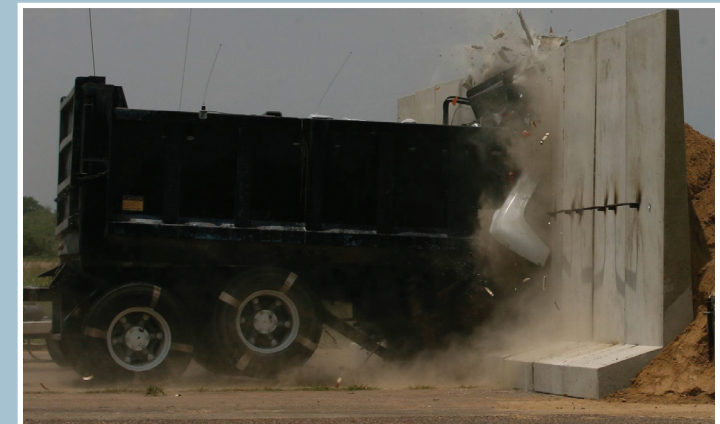
Force Protection - Above, a large threat vehicle impacts a double-wall vehicle barrier system.
