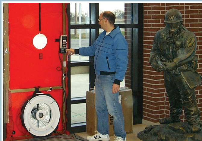
Blower Door Test - Leakage rate testing for facility collective protection against chemical/biological threats.
