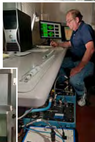
High resolution eddy current array probe technology for high-speed inspection of steam generator tubing. ▶
