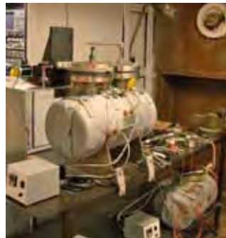
▲ Argonne's Ultrasonic Under Sodium Viewing Test Facility for liquid metal fast reactors can sustain high temperature and reactivity with most metals, providing nondestructive, real-time and in situ ranging and imaging.
