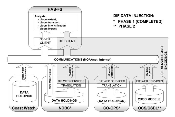
Figure 5.1 HAB-FS Data Flow Diagram
