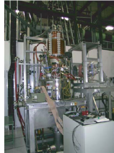
Developmental depressed collector gyrotron installed in new "socket"
