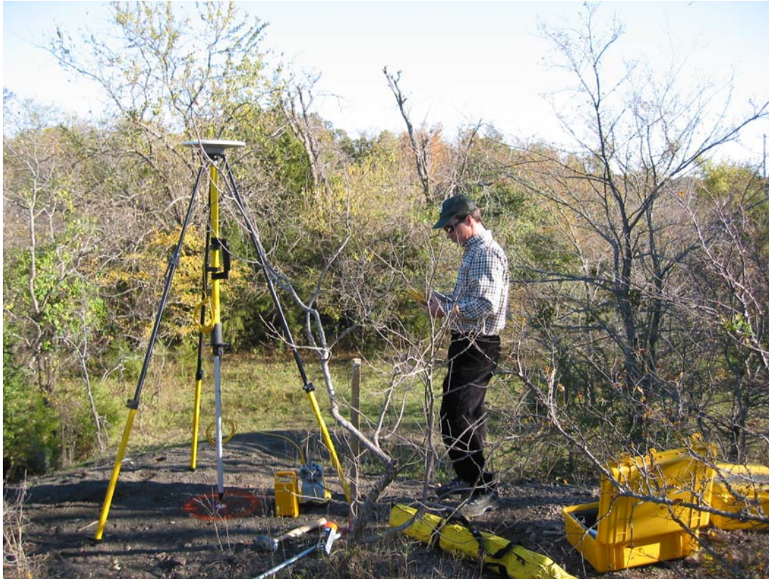
Figure 9. –Real-time Kinematic GPS Survey Activities: Setting up a Base Station on top of the Waste Dump at the Rock Island No. 7 Airshaft, November, 2002.
