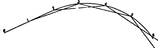
Fig. 1—Method of Measuring the Middle Ordinates of a Curve
