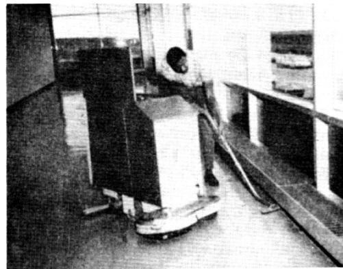
Figure 13. 30" Automatic Battery Powered Dry Pickup Machine.
