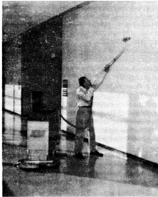
Figure 11. Automatic Battery Powered Floor and Wall Dusting Machine.
