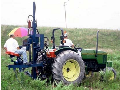
Figure 7. A tractor-mounted cone penetrometer is being used to evaluate soil density on a Kentucky surface mine.
