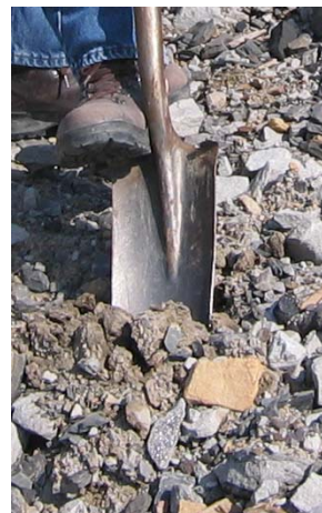
Figure 6. A spade can be used to estimate mine soil density and the need for ripping. Depth of penetration when applying foot pressure and a rocking motion is an indicator of soils’ capability to support trees that will survive and grow into commercial products (see Table 1). This long-nosed drain spade was able to penetrate spoil easily; this area should be able to grow trees successfully without being ripped.
