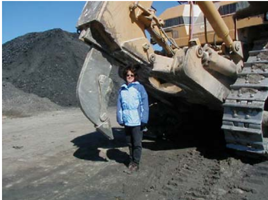
Figure 3. A single-shank ripper is capable of ripping the soil to a depth suitable for forest trees when attached to a large dozer.
