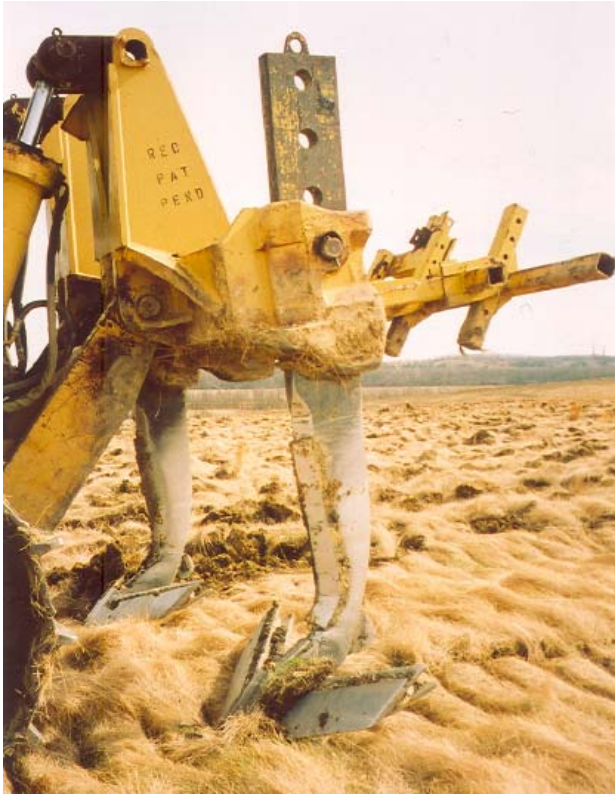
Figure 5. This ripper with a plow attachment can be used to loosen soils that do not contain large rocks and boulders. The “wings” on the ripper blade will loosen soils located beside ripping trench.
