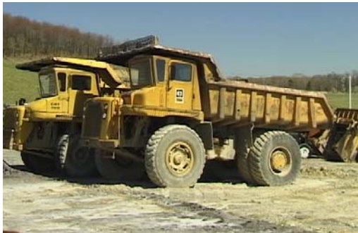
Figure 1. Even when empty, haul trucks can weigh 50 - 100 tons or more; this weight exerts force where tires meet the land surface, causing severe compaction of mine soils. Loaders, dozers, and other heavy mining equipment also cause compaction that hinders tree growth when operated on surface soils.
