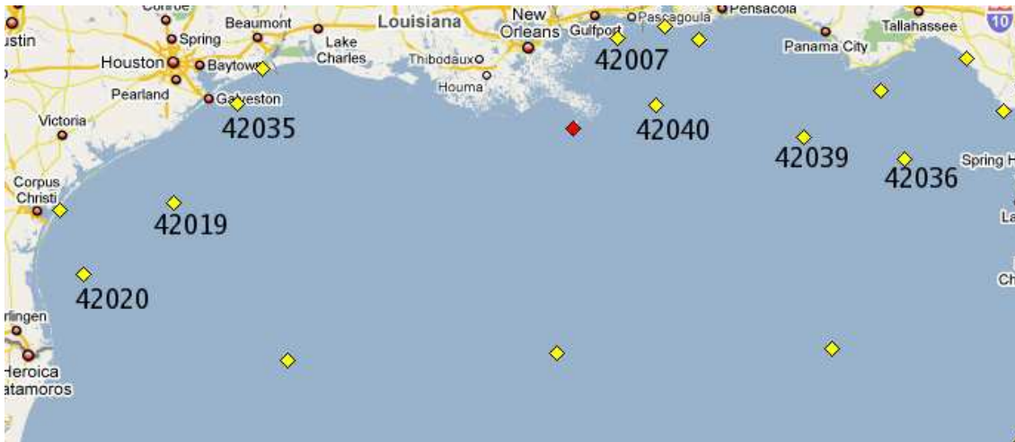
Fig. 2.1 : NDBC buoys for climatology study. The NDBC met/ocean buoys are identified by yellow diamonds and the stations used in this study are labeled by their unique 5 character long ID numbers
