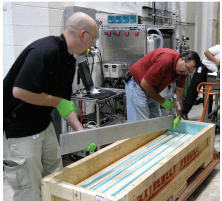
FIGURE 2: Senior Reactor Operators Bill Mueller and Jeff Burmeister remove prototype NBSR shim arm for examination.
