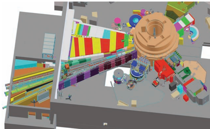
FIGURE 4: Design drawing showing the planned layout of the confinement building and D-wing post-outage in early 2012 with the new guides installed. MACS (analyzer not shown) is in place at BT-9.
