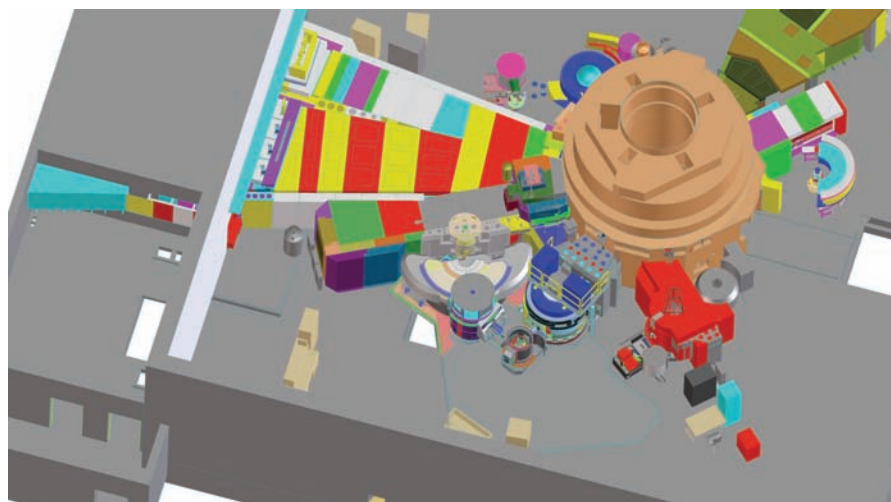
FIGURE 3: Design drawing showing the current layout of the confinement building and D-wing (on the left). The MACS at NG-0 (kidney-shaped analyzer) and the Double Focusing Triple Axis spectrometer at BT-7 to MACS' right can be seen in the center of the figure. To the right of BT-7 is the residual stress facility at BT-8, and beyond that (circular gray object) is BT-9, to which MACS will be moved.
