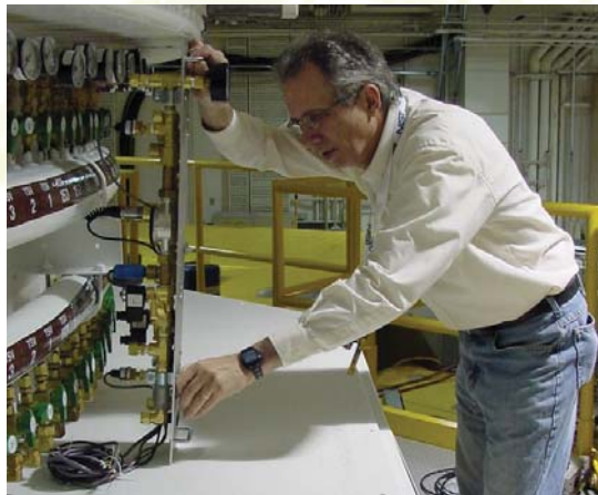
FIGURE 3: Engineer Tony Norbedo places a test module designed to monitor thermal shield performance.
