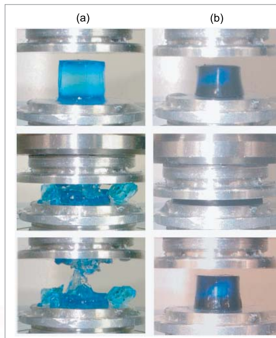
FIGURE 1: Pure PAMPS gel breaks down under compression at 40 % by volume (a), but the toughest DN-gel regains its size and shape after 90 % compression by volume (b). (Reproduced with permission from Ref. 1.)
