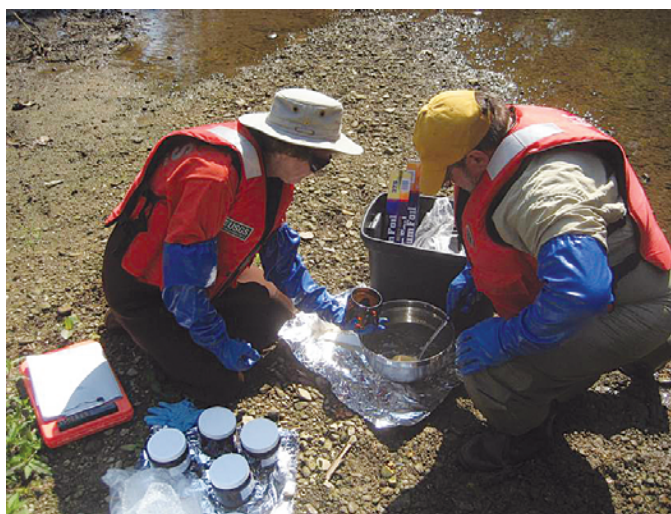
Figure 5. U.S. Geological Survey and Pennsylvania Department of Environmental Protection scientists processing a streambed-sediment sample in the field.
