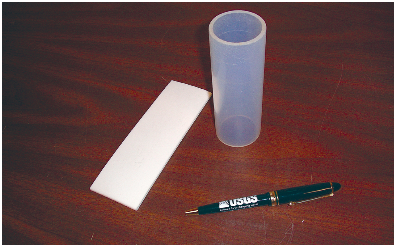
Figure 4. Teflon cylinder and Teflon wafer used to collect streambed-sediment samples.
