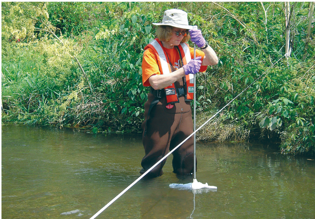
Figure 3. U.S. Geological Survey hydrologist collects a water sample for analysis of contaminants of emerging concern using a DH-81 sampler fitted with Teflon adapter, Teflon nozzle, and Teflon 1-L bottle.
