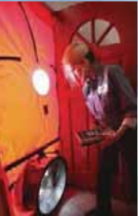
Left: Roseann Mitchell, of the Community Action Agency, checks air-flow readings as part of a blower door test assessment, in San Francisco. (AP Photo/Ben Margot)
