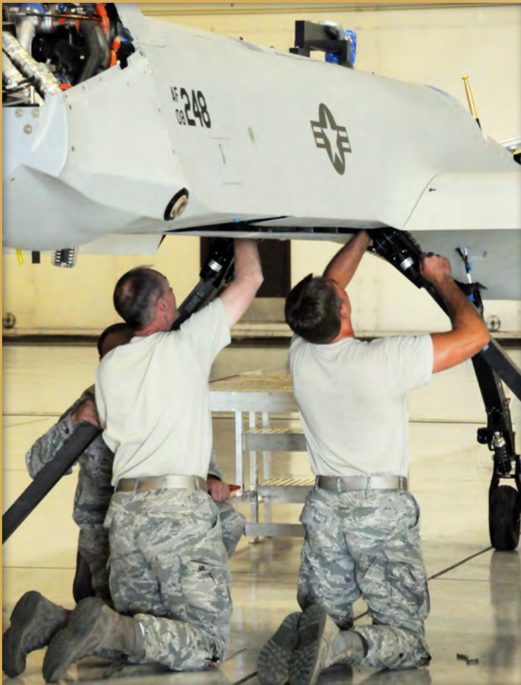
(Left) Col. John Dougherty, the 119th Operations Group commander, points out locations on a training flight map for Maj. Gen. David Sprynczynatyk, N.D. adjutant general, right, in the 119th Launch and Recovery Element (LRE) operations area at the Grand Forks Air Force Base, N.D. (Above) 119th Aircraft Maintenance personnel assemble one of the first Launch and Recovery Element (LRE) MQ-1 Predator aircraft at the Grand Forks Air Force Base, N.D.
