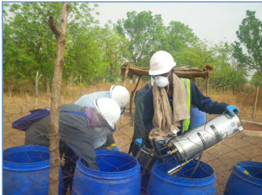
Spray operators conducting the Progressive Rinse. Barrel #1 is for dumping, Barrel #2 is for fetching clean water to shake spray can with, Barrel #3 is for dumping for a second time... and so forth
