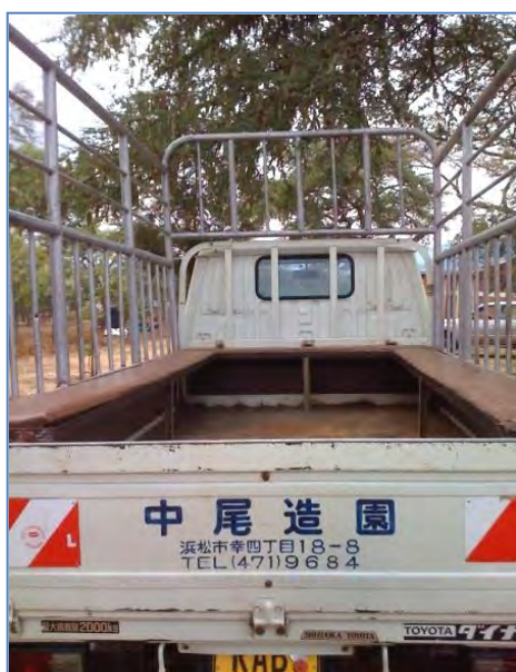
Truck retrofitted with side bars and benches both for SO safety and comfort
