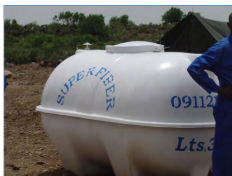
Polythene tank used as secondary storage of DDT effluent waste
