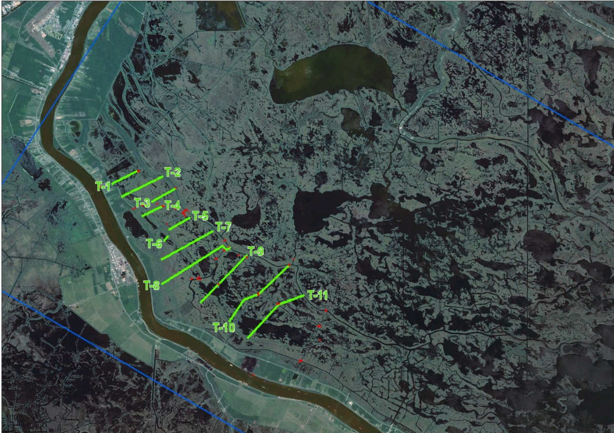
Figure L2.1: Surveys contract by the USACE to assist in Hydrodynamic modeling analysis of the White Ditch project area.
