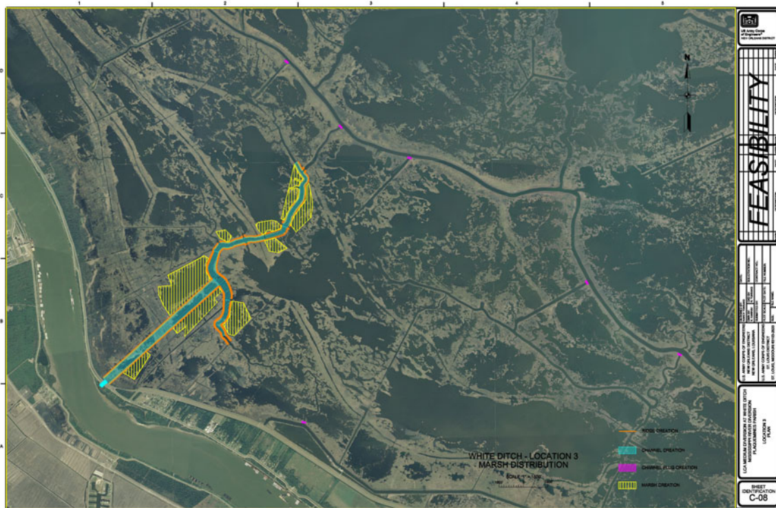
Figure 2. Tentatively Selected Plan for Medium Diversion at White Ditch Feasibility Study, a 35,000 cfs diversion near Phoenix, Louisiana.
